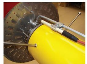
The unique spider head assembly offers the user high turn down ratios. It was initially designed to be fired when using fuels with high burning velocities such as Propane or Hydrogen. Unlike the split head, the fuel is introduced after the diffuser plate enabling the flame to establish good retention whilst maintaining excellent mixing. Limpsfield will design and engineer the correct solution to suit your application.
